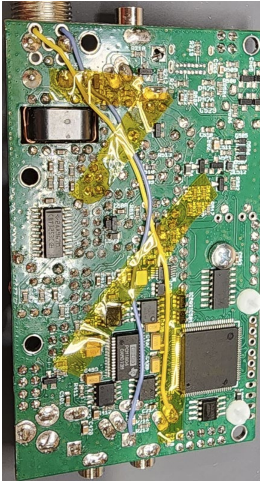
Figure 6 – TIP and RING signal wire routing on bottom side of the board.
